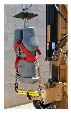
7.4 The shackles or manufacturer specified hardware shall be attached from the suspension lines to the two specified hip picks. The test connection equipment (shackles, slings, carabiners, cable, chain, etc.) shall load directly on the two points of the harness so as NOT to bind or cause additional leverage on the picks.
